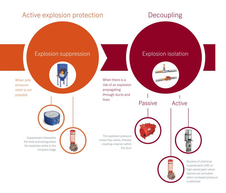
the duct. Active isolation includes high-speed gate valves or barriers of chemical suppressant, which are activated at the time the increased pressure is detected.
