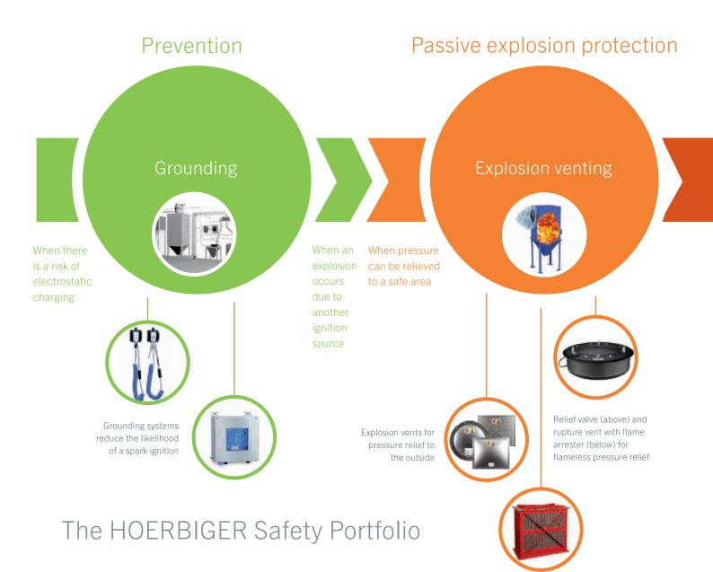
A range of flameless venting solutions are also available to allow venting indoors in certain situations. These either employ an essentially maintenance-free relief valve, which closes automatically after the pressure has been relieved, or a conventional rupture vent, which is combined with a flame arrester. Both products prevent flames from escaping the facility.
